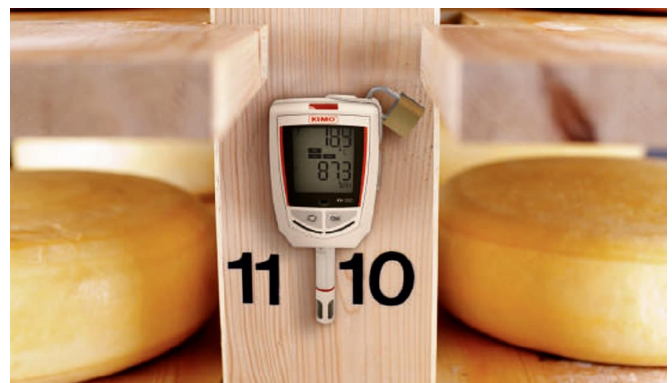
Relative humidity and temperature control in a maturing cellar using a KH 220 mounted onto a plate and secured with a padlock as part of a mapping process
